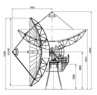
Probecom 13 Meter Cassegrain antenna can deliver superior performance, with linear and circular polarization, for Multi-bands, L,S,X Tx/Rx sat communication applications such as Broadcasters, Service Providers, GSM operator, Satellite operator, Military and Government Agencies, FreeLands or Rescue Organizations.
