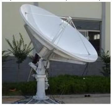
**Probecom 2.4 Meter Ring focus antenna** can provide Tx/Rx 2-port feed in switchable linear & circular polarization for C-band, 2.4m Ku band can only be for linear polarization. Delivering exceptionally high performance for transmit/receive applications.
