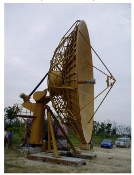
Probecom 9.0 Meter ringfocus antenna can deliver superior performance for C-band and Ku-band transmit/receive sat communication applications such as Broadcasters, Service Providers, GSM operator, Satellite operator, Military and Government Agencies, FreeLands or Rescue Organizations.
